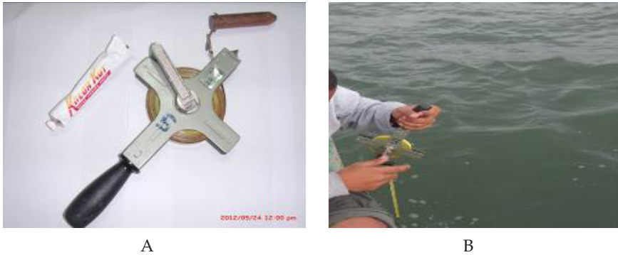
Fig. 1. A. Sounding paste and tape. B. In situ measurement of water depth using sounding paste and tape
