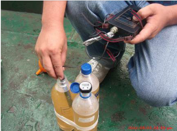
Fig. 5. In situ measurement of pH, temperature and salinity of ballast water
